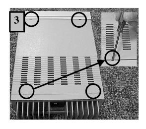
**REMOVE COVER** by prying Rear Bezel and Front Panel away from Cover in four places as shown. Then lift Cover off unit.
