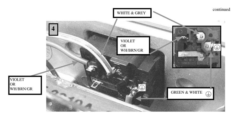
**REPLACE MODULE** with P/N 5185-1346. Before soldering perform "TEST FOR LOOSE AC MODULE" as shown in picture above. This will confirm that the new Module is secure. Solder wires and **REPLACE FUSE**.
